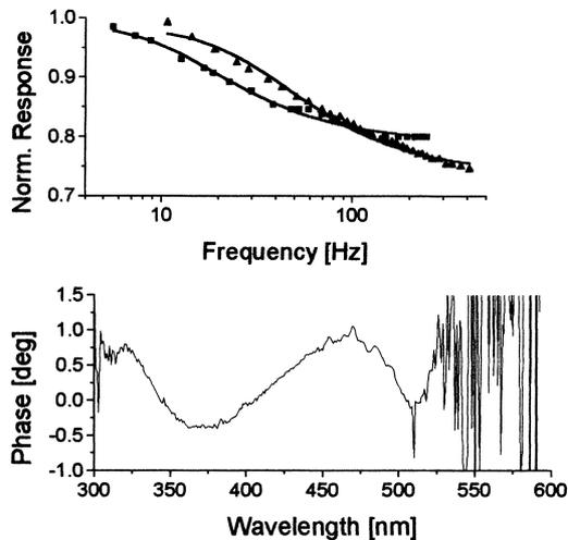
Fig. 5. Top: normalized photocurrent vs. chopper frequency for the thick (PPV/PMA)<sub>32</sub> devices. Triangles denote the results obtained for the excitation wavelength  $\lambda_{exc} = 500$  nm, squares refer to  $\lambda_{exc} = 350$  nm. Bottom: Phase angle of the spectrally resolved photocurrent.
