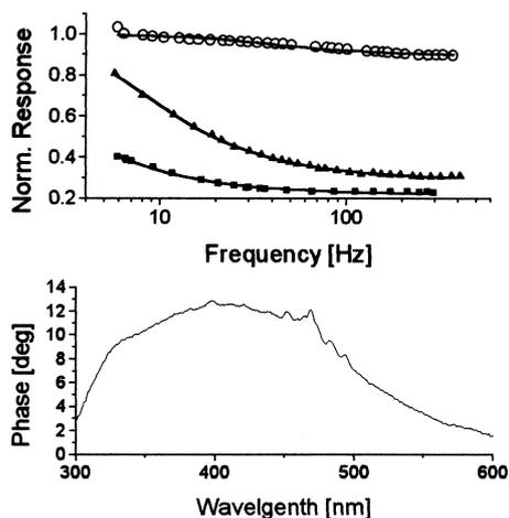
Fig. 6. Top: normalized photocurrent vs. chopper frequency for the thick (PPV/C<sub>60</sub>(OH)<sub>24</sub>)<sub>32</sub> devices. Open circles denote the results obtained for the excitation wavelength  $\lambda_{exc} = 580$  nm; triangles refer to  $\lambda_{exc} = 500$  nm; squares refer to  $\lambda_{exc} = 350$  nm. Bottom: Phase angle of the spectrally resolved photocurrent.
