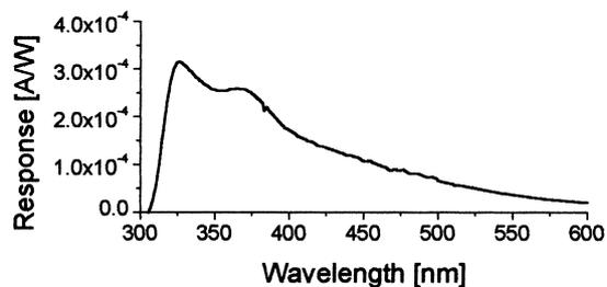
Fig. 3. Photocurrent action spectra of the thick  $(\text{PPV}/\text{C}_{60}(\text{OH})_{24})_{32}$  devices.
