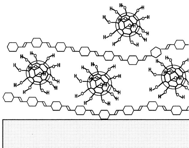
Fig. 1. Composition of the PPV- $C_{60}(OH)_{24}$  ISAM films on a molecular level. This is a “magnification” of the schematic bilayer structure. The grey area represents the substrate.
