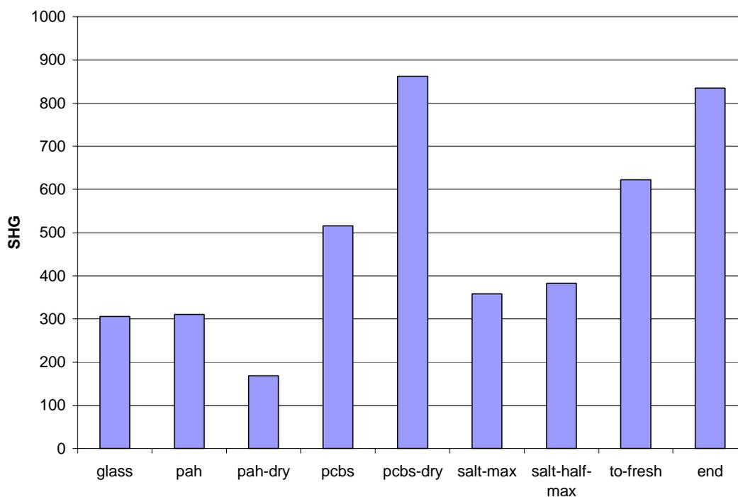
**Figure 5. Final values of the *ex situ* SHG signal for different deposition steps. Immersion in salt solution results in a rapid decrease in signal, which is restored when the sample is immersed in deionized water.**
