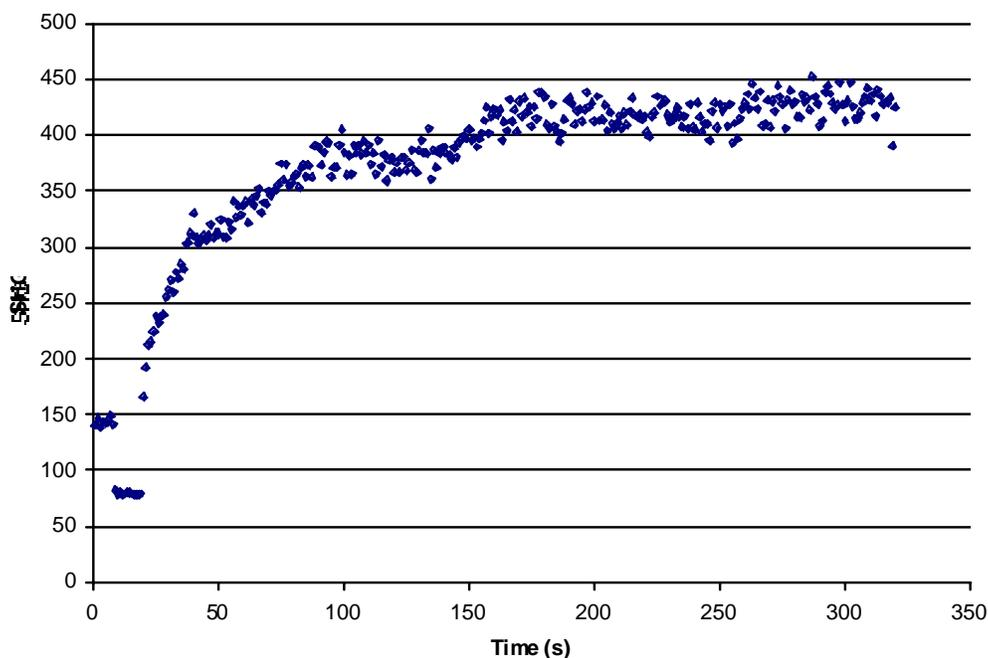
**Figure 6. The SHG signal as function of time during deposition of procion red on PAH.**
