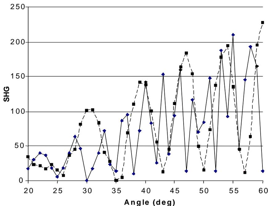
**Figure 2. The SHG as a function of incident angle for a PAH/PCBS sample. The solid and dashed lines represent the sample in water and in air, respectively.**
