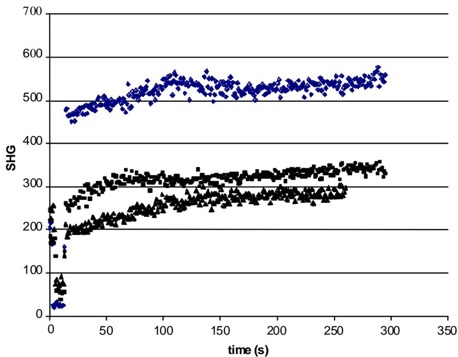
**Figure 4.** SHG signal as function of time during PCBS deposition on PAH for low concentrations of PCBS. The concentrations, top to bottom, are 0.5 mM, 0.05 mM, and 0.0025 mM.
