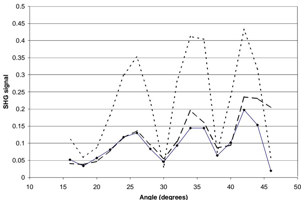
**Figure 1. The second harmonic signal as a function of incidence angle. The solid line represents the glass slide, which has some SHG signal due to the fact that the interface is non-centrosymmetric. The dashed and the dotted lines represent the same slide after depositing PAH and PCBS layers, respectively.**
